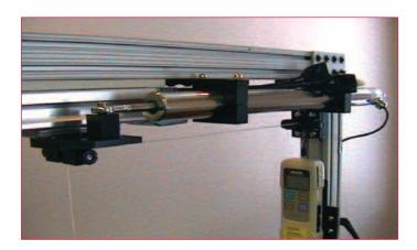
Figure 1. cyberDERM PEEL tester
