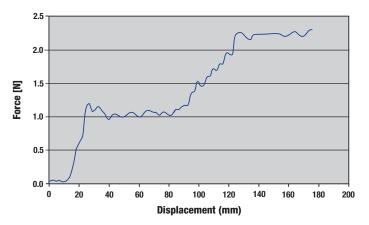
Figure 3. Peel Test Results-Subject #1
